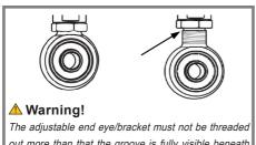
out more than that the groove is fully visible beneath the lock nut. This is maximum length. After adjusting, make sure that the lock nut is tightened (30Nm).
