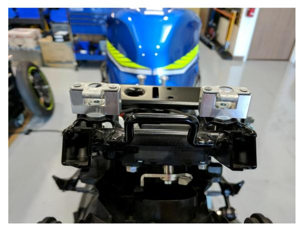
Install the Rear flat bottom brackets on subframe then screw on dzus plate
