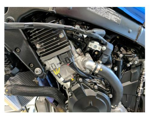
Install CNC brackets into metal bracket on each side of the bike and use washer and lock nut to secure.
