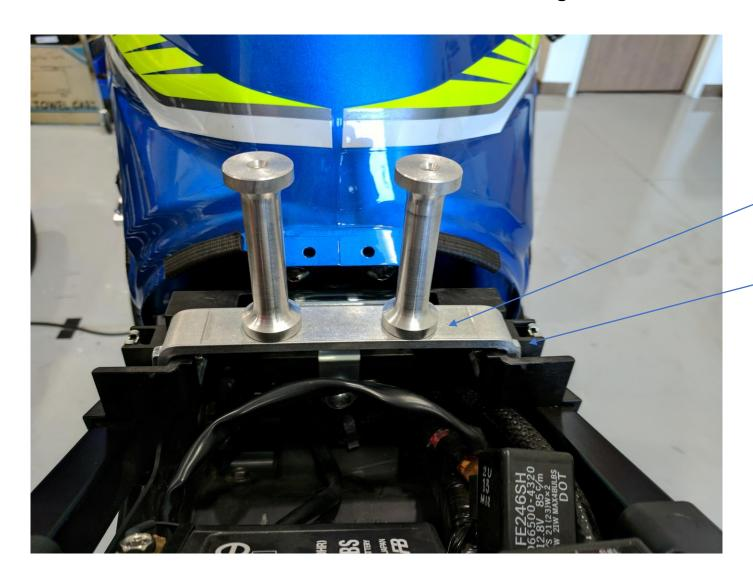
Attach Seat Post to bracket with Supplied Bolts
