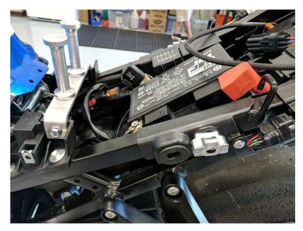
Install CNC brackets to left and right side of subframe (these have a neck to go into the hole) install dzus bracket
