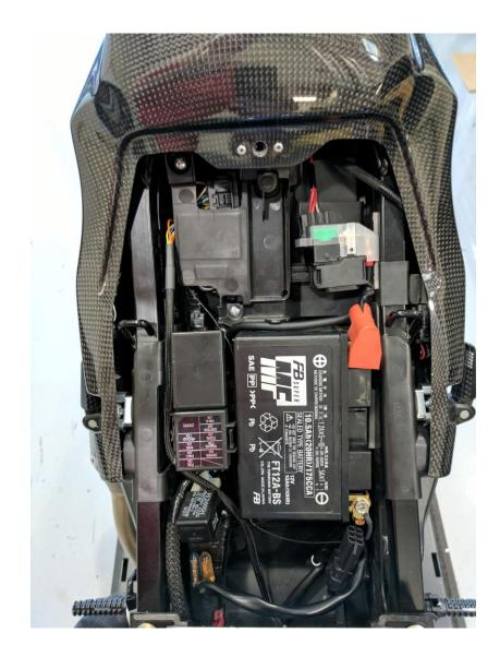
Slide over tail unit and use x4 dzus to install Then fasten seat to the seat pan with provided locking nuts
