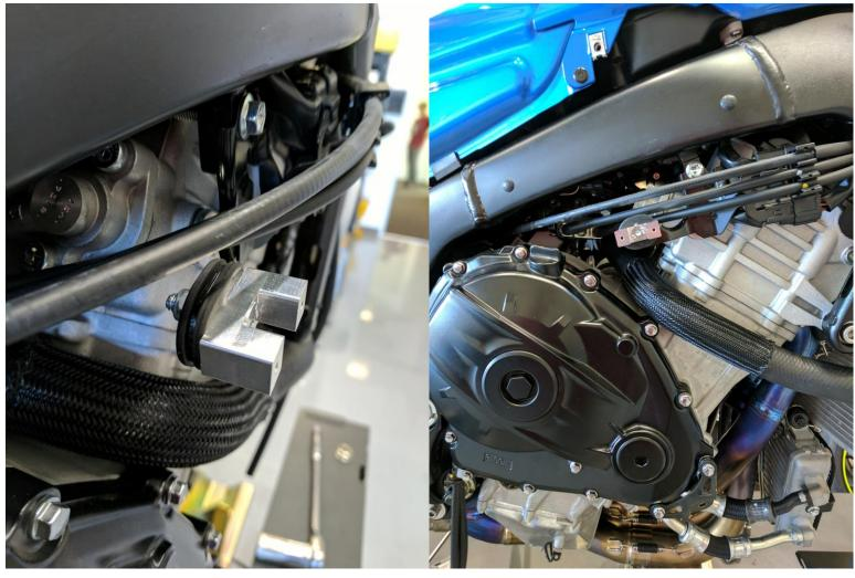
Install left bracket using OEM side stand Bolts
