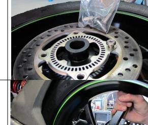
Carefully put the wheel into the swingarm and slide in the axle bolt provided.
