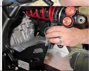
Therefore mount the pull rod to the frame with the correct nut and bolt, make sure you hold the nut whilst tightening. Use manufacturer recommended torque settings.
