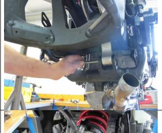
The shock absorber should now be completely separated from the swingarm.
