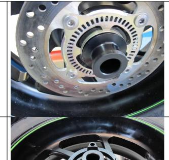
Rlace the distance ring on the brake disc pick up points.
