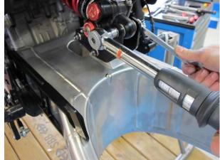
Now tighten all bolts connecting the link and the swingarm to the manufacturer torque settings. Make sure you hold the nut whilst tightening.
