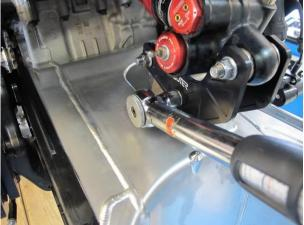
Now fix on the mudguard using the three bolts provided. Tighten the Bolts according to the value in the Suter-Torque-Table.
