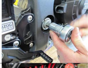
Install the shock absorber, the pull rod and the link.
