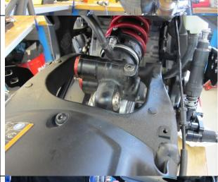
Remove the speed sensor. Make sure that it won't get damaged when rebuilt.
