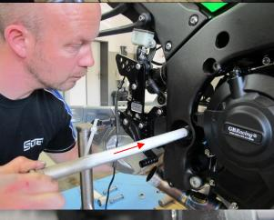
The swingarm should fit tightly between the frame and the bush provided.
