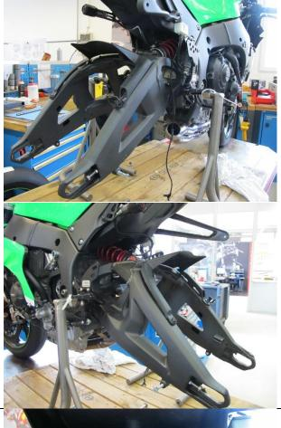
Remove the link bolt from the shock absorber.
